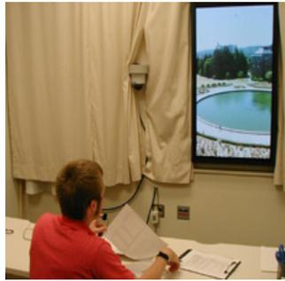
(a) The plasma-display window covered up the same-sized real window used in the window view condition. The recording camera can be seen through the drapes to the left of the plasma display. The drapes were pulled across the entire wall for the blank-drapes condition.
